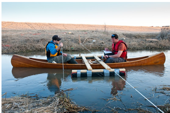
Above: Marc St.Laurent and Mike Morris complete a river flow measurement downstream of siphon outlet near the floodway.
